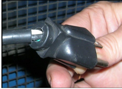
Figure 1-1.--Cord with Damaged Outer Jacket
