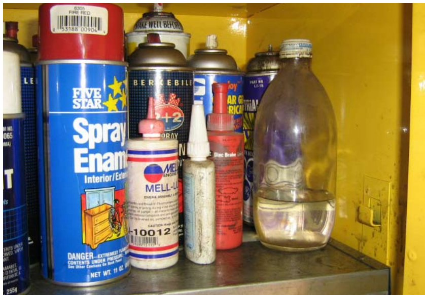
Figure 3: An unlabeled bottle in a storage cabinet for flammable chemicals risks misuse or consumption.
