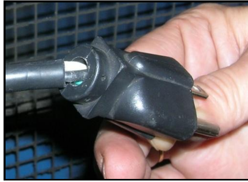
Figure 1-1.--Cord with Damaged Outer Jacket
